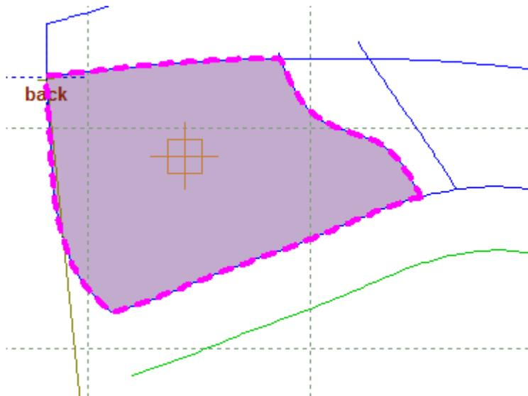
4. Before ending the process you can select more parts; just position the cursor again in the middle of the desired lines.
