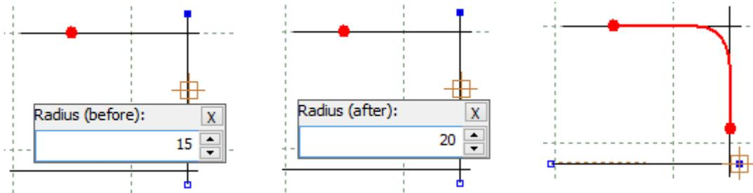
**Arc on next** - Select this option to apply the type of corner **Arc** in the intersection between the selected line and the next selected line.
