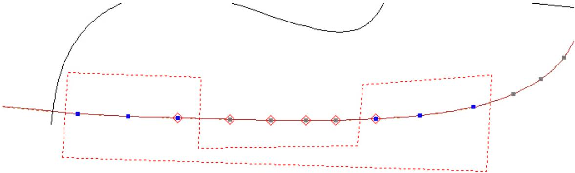
2. select **Fittings Grading Connection** from the **Advanced** options on the **Grading** menu. The smoothing connection handles will appear inside blue diamond shapes.
