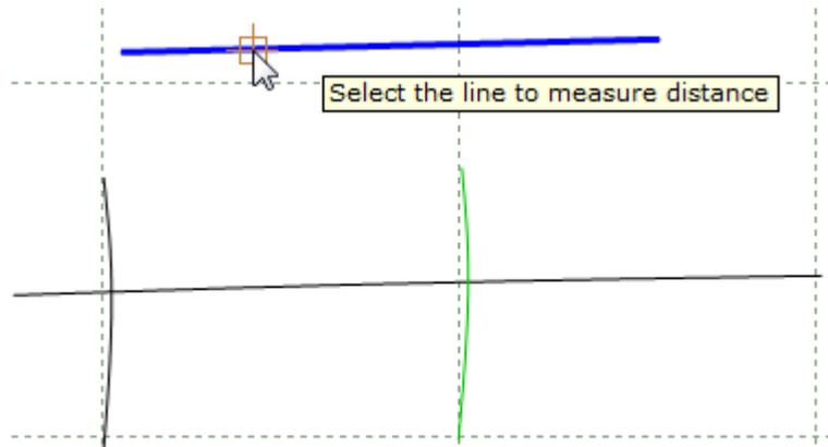
10. If we increment the "line to measure distance", the distance between the green line and the master line will be automatically readjusted.
