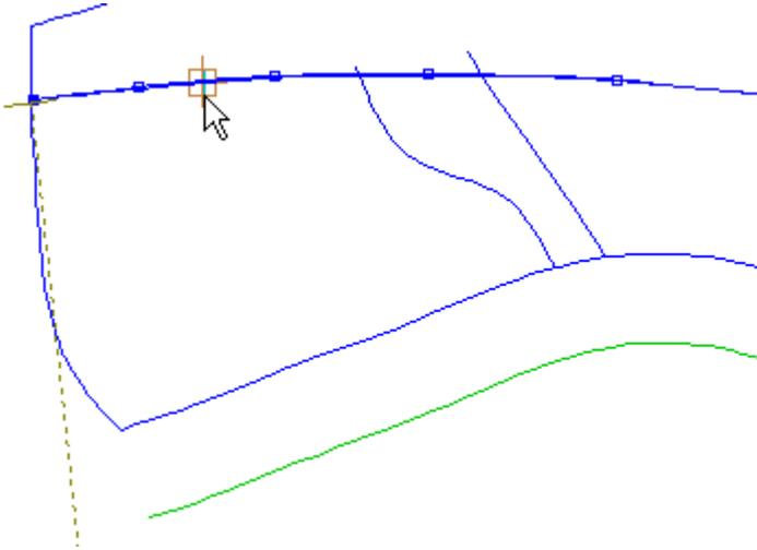
3. Continue to select lines going in the same direction. The direction is not important as long as within each part you move in the same direction.
