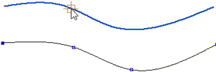
The anchor line turns yellow. Any edits done to the master line are reflected in the anchor line
