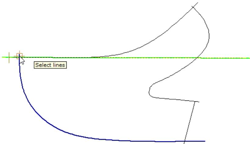
7. It's possible to select just a part of the line, just keep the left mouse button pressed over the line and drag, from the start point until the last point you want to select.
