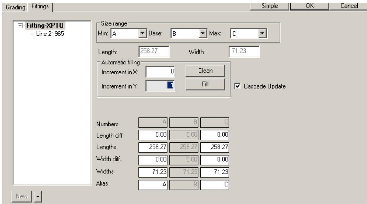
6. lines being affected by the fitting will turn into a ruby colour, the constrained control points will be displayed inside red diamond shapes and the unrestricted control points into blue.
