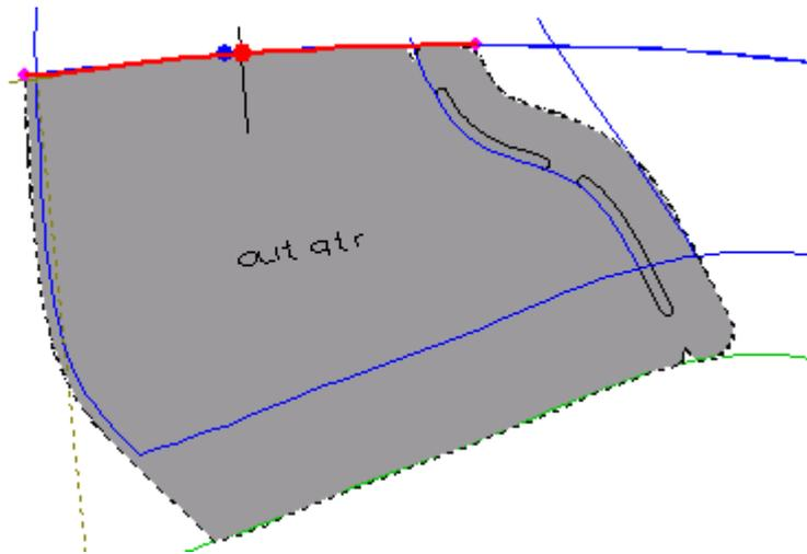
2. Press **Shift** and move the cursor towards the line that defines the cut position. The cut cursor will
