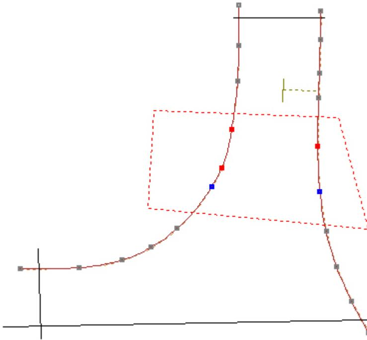
2. select **Grading Connection** from the **Advanced** options on the **Grading** menu. The smoothing connection handles will turn into a light blue.
