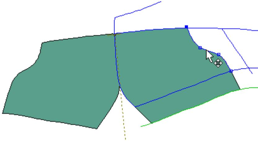
2. Select **Replace Lines/Reflection** from the **Replace Lines** options of the **Parts** menu.
