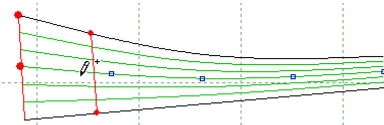
8. It's possible to change the parameter and its position by dragging the red points over the lines (middle red point to change position, top red point to change parameter), or by change the values in the **Tool Options**.
