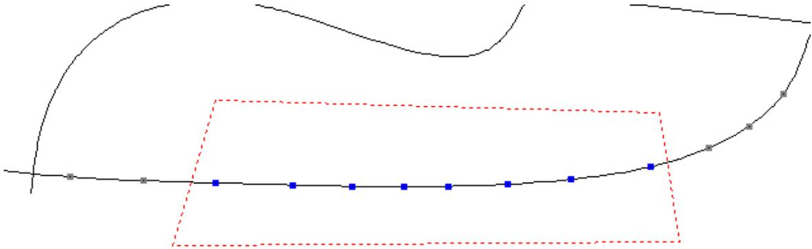
2. if the fitting is to be applied only to a section of the lines then select the affected area by doing a net selection while pressing **Shift**.
