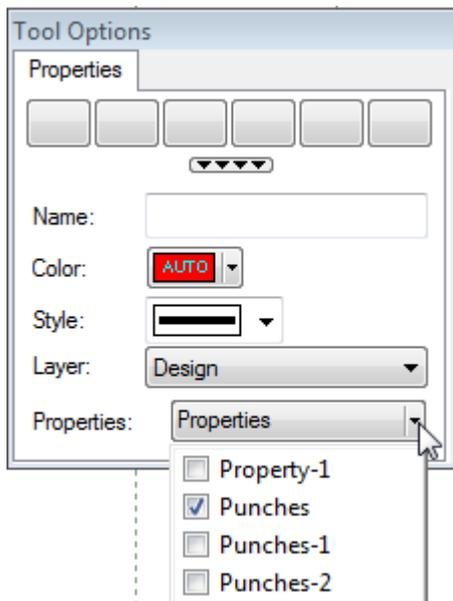
3. It's possible to insert a name, change the colour, the style, the layer and assign one or more properties, to add new property go to **Preferences, Default Properties** tab.
