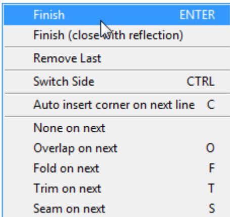
7. Select **Finish** to complete the part. The part can also be finished by pressing the **Enter** key or clicking the middle mouse button.
