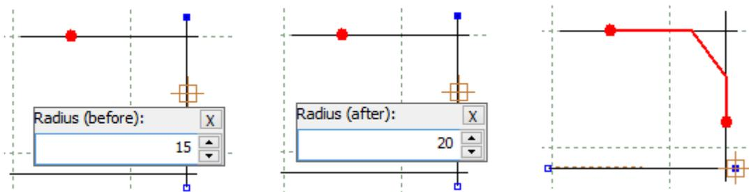
**Bezier on next** - Select this option to apply the type of corner **Bezier** in the intersection between the selected line and the next selected line.
