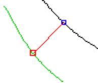
To release this constrain, you can either do a right click and select Clear distance from the contextual menu, or approach the line with the mouse cursor and "Cut the line". When the mouse cursor is placed over the connector line, will change and appear like a scissors, just do a right click to release the point.
