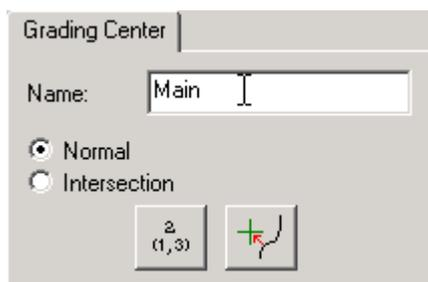
3. Move the cross hairs to the position required for the grading centre and press the left mouse button.
