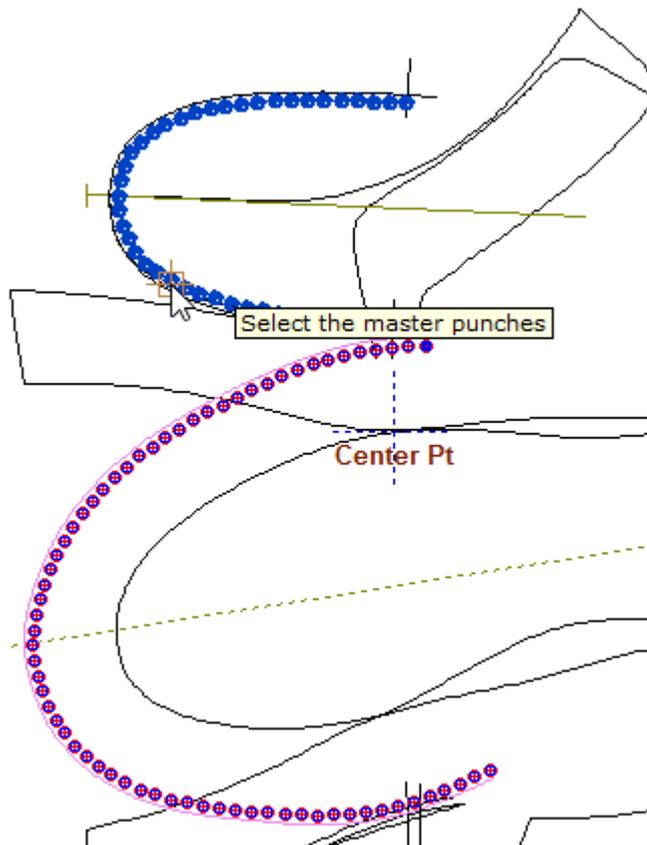
5. The new punches will be automatically rearranged based on the masters.
