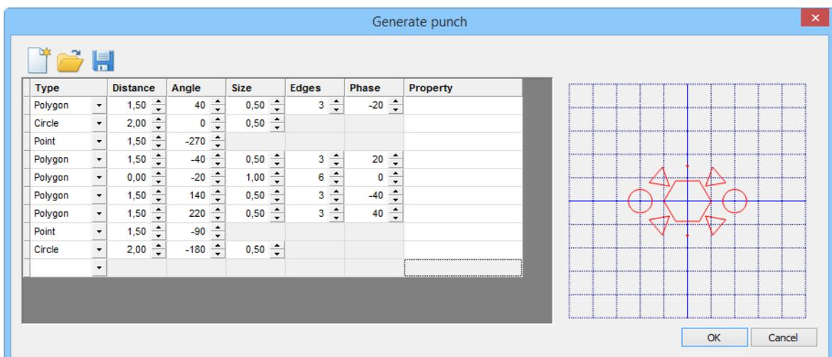
5. To easily identify which type is shown in the preview, just move the mouse cursor over the preview and the Type and parameters will be highlighted.
