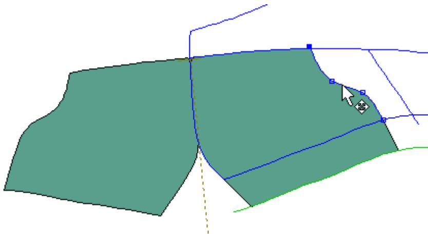
2. Select **Replace Lines on Reflection** from the **Replace Lines** options of the **Parts** menu.
