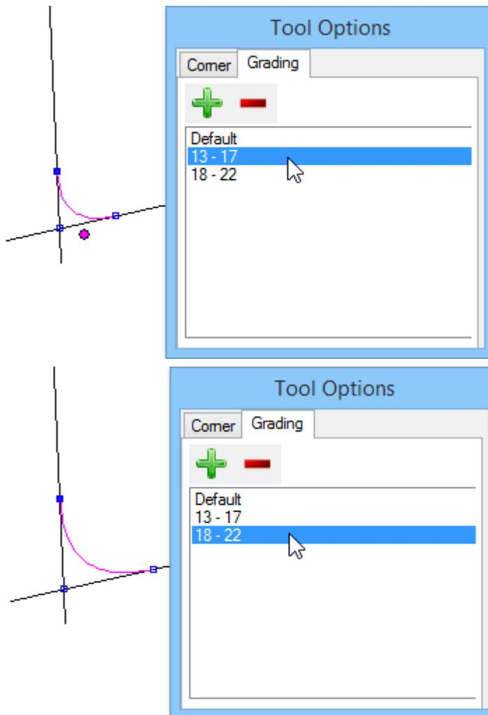
7. To remove a grading rule, select it and press the button
