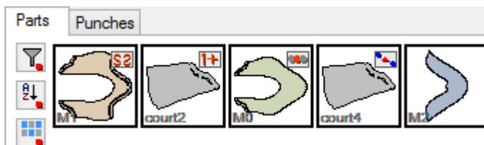
Besides the graphical representation of the part, containing outer boundary and all the elements that could be included on a part (markers, notches to name a few), there are auxiliary symbols appearing on the top right corner of the thumbnail.
