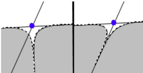
**Oblique** - A notch with the base of the triangle placed on the line it is created from. Oblique notches can only be applied using the intersection option.
