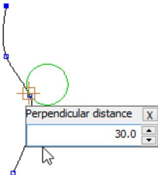
**Automatic distance** - The diameter is controlled by the mouse position.
