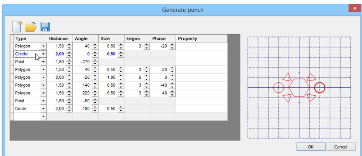
7. When finished, press Ok and the punch will be applied.
