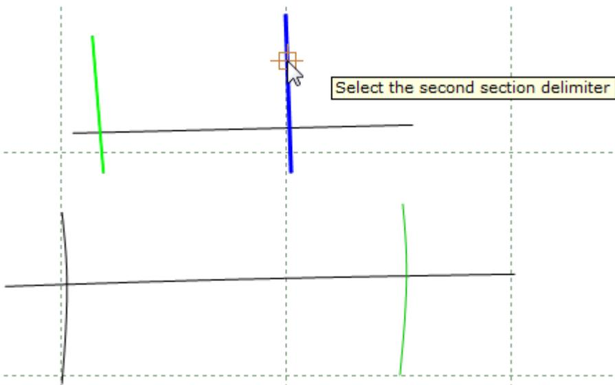
17. The new section is created equal to the main section, if the main section is changed, the new section will be readjusted, to ensure that the both sections have exactly the same length.
