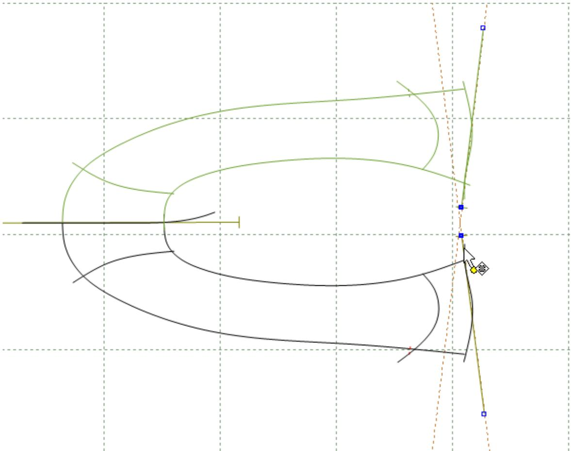
Activate the axes. To activate the axes you can go to **Operations - Mirror - Active Axis** or press **CTRL+E**, after Axes selection.
