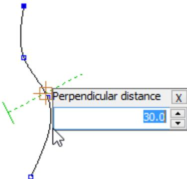
**Automatic distance** - The distance is controlled by the mouse position.
