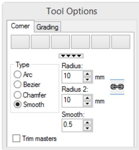
**Type** - Select the corner type between **Arc**, **Bezier**, **Chamfer** or **Smooth**
