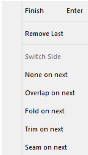
7. Select **Finish** to complete the part. The part can also be finished by pressing the **Enter** key or clicking the middle mouse button.
