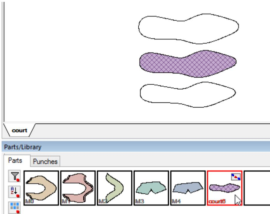
5. To define the grading for each part size, in the **Parts** toolbar, do a right mouse click over the part and select Properties.
