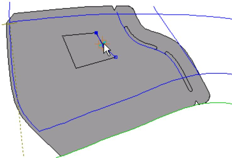
4. Define the rest of the boundary of the hole going in one direction.
