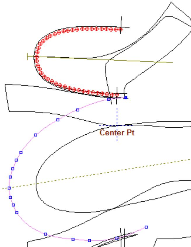
2. Select **Punches** from the Operation menu or press **F9**. The last punch configuration used will be automatically applied to the line.
