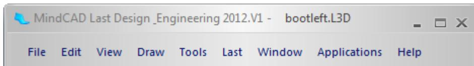
Almost everything in **MindCAD 3D Last Design & Engineering** can be accessed through the main menu. This is shown in the picture above and is displayed at the top of the **MindCAD 3D Last Design & Engineering** screen.
